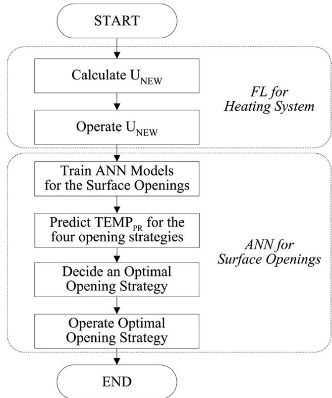
Fig. 5. Flow of the 3rd algorithm.
