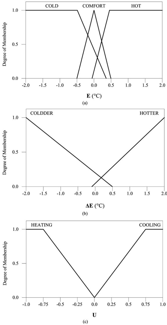
Fig. 6. (a) Membership function plots of E (1st input), (b) membership function plots of ΔE (2nd input), (c) membership function plots of U (output).
