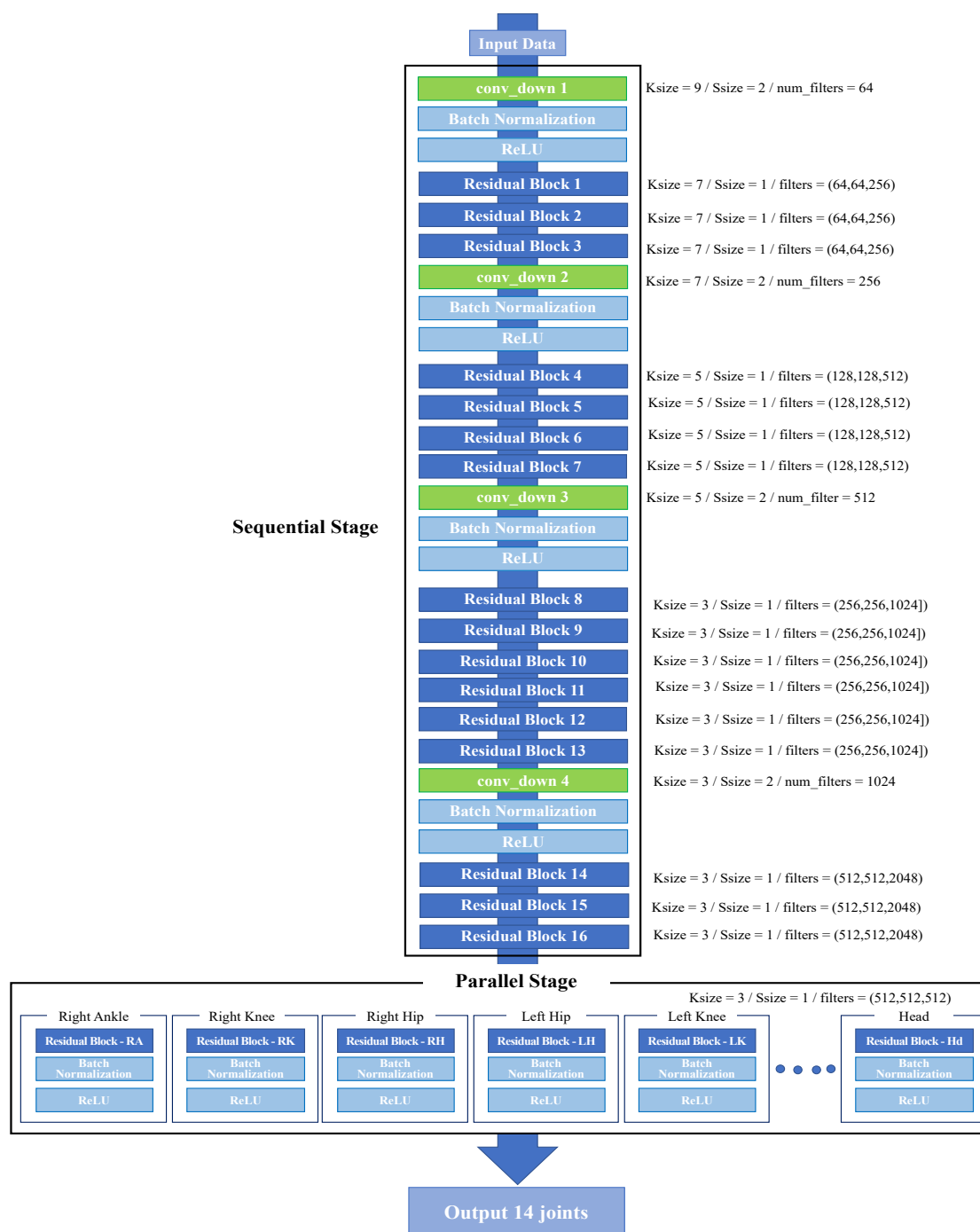
Figure 5. The structure of proposed deep neural network (DNN) model for activity estimation.
